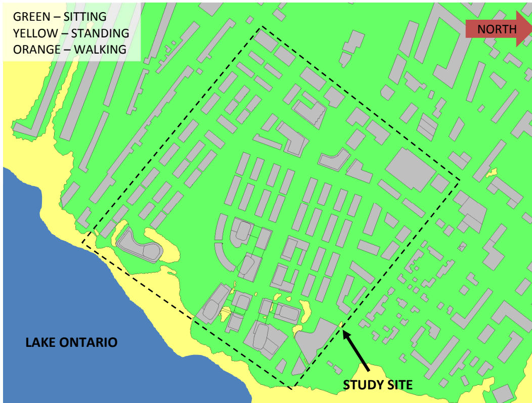
FIGURE 3: SUMMER – GRADE-LEVEL PEDESTRIAN WIND CONDITIONS FOR PROPOSED DEVELOPMENT
